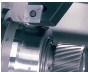
TiAlN coated CBN grade BNC200 for high speed continuous to medium interrupted cutting
